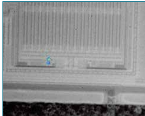
Overlay of thermal emission (in pseudo color and after thresholding) on the thermal background image.
